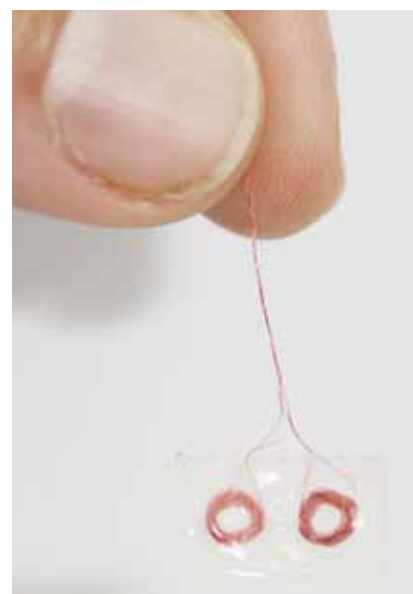
The swimming tail that propels the capsule endoscope
